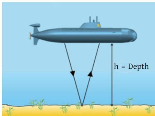
Submarine measuring the depth from the echo time of a sonar.
